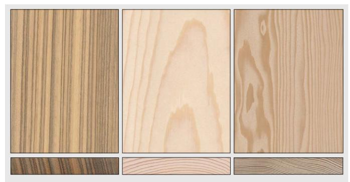
Reading the grain: note the appearance of the face grain of these three boards, as well as their corresponding endgrain surfaces beneath. On the left, Beli (*Julbernardia pellegriniana*) is almost perfectly quartersawn, resulting in a straight, narrowly spaced, and uniform grain pattern. In the middle, Ponderosa Pine (*Pinus ponderosa*) is flatsawn, resulting in a
