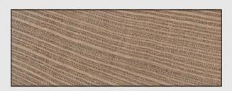
The rays seen in this  $1 \times$  endgrain view of Lacewood (*Panopsis spp.*) are so large and prevalent, they could easily be mistaken for growth rings.
