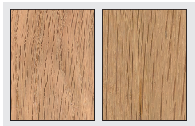
Black Oak ( Quercus velutina ) is pictured on the left, and exhibits very short rays, indicative of red oak species. The image on the right shows the longer rays that are characteristic of flatsawn sections of the white oak species—in this case, Swamp Chestnut Oak ( Quercus michauxii ).
